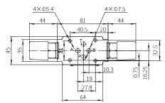
Valve fixing screw M5-10.9 grade GB/T70.1-2000
