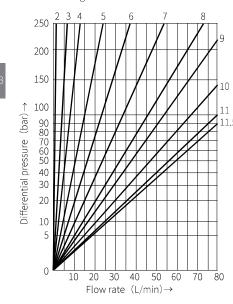
△p-qv characteristic curve Z2FS6... -4XJ/1QV Throttle setting in turns
