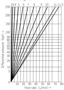
△p-qv characteristic curve via check valve (throttle valve closed)
